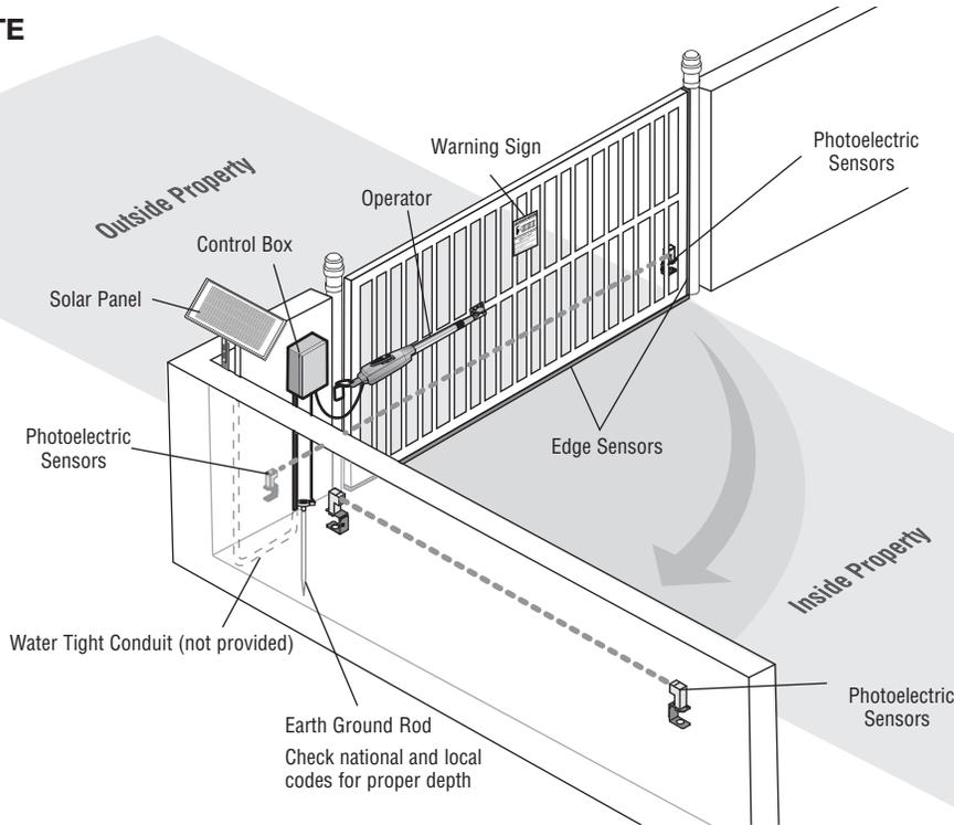
**NOTE:** One or more non-contact sensors shall be located where the risk of entrapment or obstruction exists at either the opening or closing direction. Care shall be exercised to reduce the risk of nuisance tripping, such as when a vehicle, trips the sensor while the gate is still moving.
